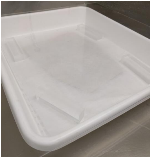
figure 9 –Albumen photo face-down in humidity chamber with smooth nonwoven polyester lightly weighted at edges with Plexiglas cubes.
