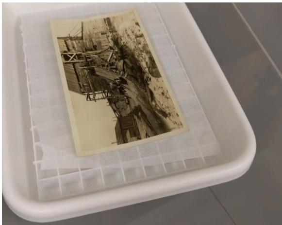
figure 8 – Gelatin photograph in humidity chamber face-up.
