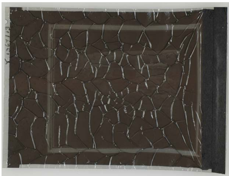
Api42 (neg. no. Y1367113) above : Degraded acetate negative. Negative has the characteristic bubbles and blisters found in degraded acetate negatives. From the collection of The CPC.
